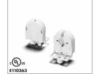
Flush-mount lampholder for T8 and T12 lamps Lamp axis: 25.5mm (1.004") Casing: PC, white, rotor: PBT GF Quick-connect twin terminals: 18AWG
