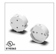
Snap-in lampholders for T8 lamps For push-fitting onto the lamp Casing: PC, white, front cover plate: PBT GF, white T110 (acc. to IEC) Quick-connect twin terminals: 18AWG Thickness of lampholder: 9.5mm (0.374") Mounting hole for #4 screw (M3) Weight: 6g, packing aty.: 1000 pcs.
