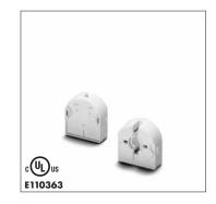
Butt-on lampholder/starter combinations for T8 and T12 lamps, with starter attachment Casing: PC, white, rotor: PBT GF, T130 (acc. to IEC) Quick-connect twin terminals: 18AWG Thickness of lampholder: 9.5mm (0.374") Rear split pins for wall thickness up to 1.2mm (0.047")
