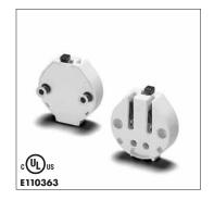
Butt-on lampholders for T8 and T12 lamps Lampholder thickness: 13mm (0.512") Casing: PC, white, frontplate: PBT GF, white
